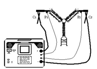
Figure 4.3: Circuit breaker connection
