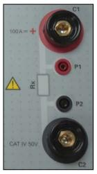
Figure 4.2: MicroOhm current and voltage terminals
