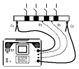
Figure 4.4: Bus bar connection
