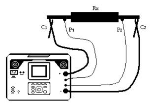
Figure 4.5: Connecting instrument to the measured device
