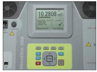
Figure 4.1: Display and keyboard layout
